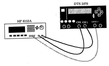
Pulse generator setup for delay measurements
