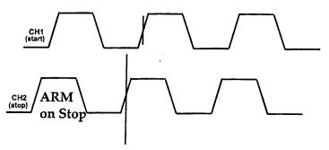
CH2 pulse leads CH1 pulse--Prop. Delay is negative
